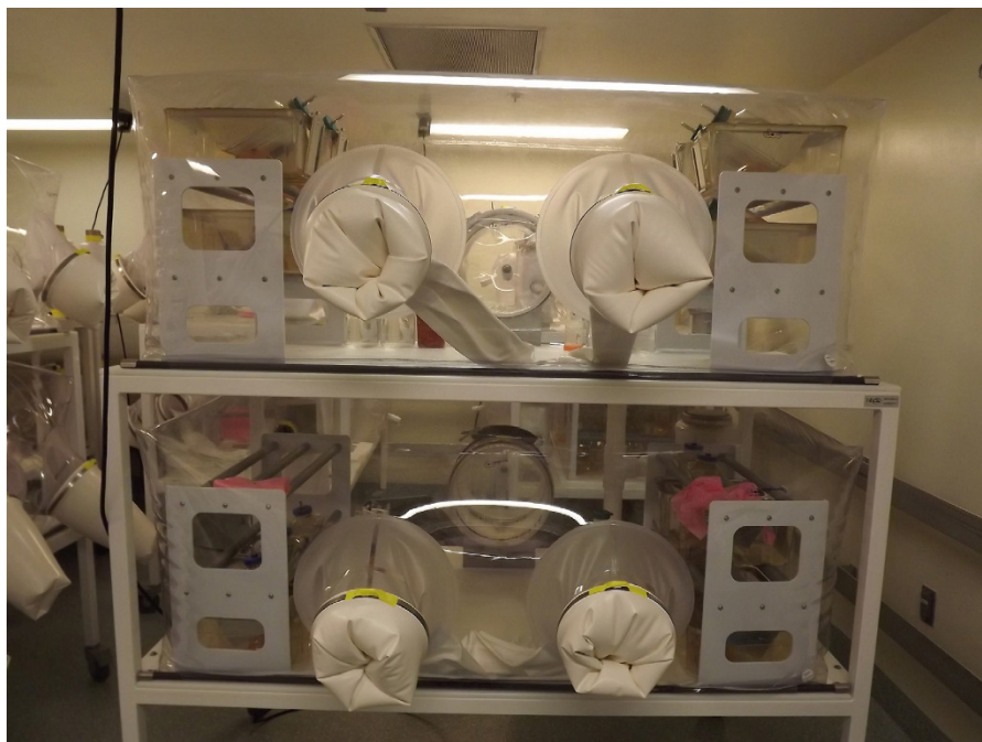
FIGURE 2 | Example of a typical gnotobiotic facility with sterile isolators. All components (such as food and bedding) have to be sterilized before being placed in each isolator, creating a strict set of requirements for maintaining gnotobiotic colonies. Image from NIAID.
